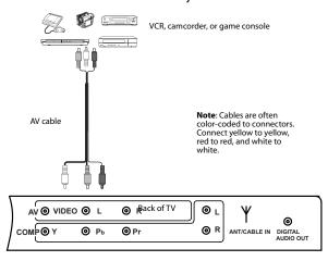
3 Connect the audio connectors of the AV cable (the red and white connectors) to the AV OUT AUDIO jacks of the external device, then connect them to the AV L and R jacks on the back of your TV.
